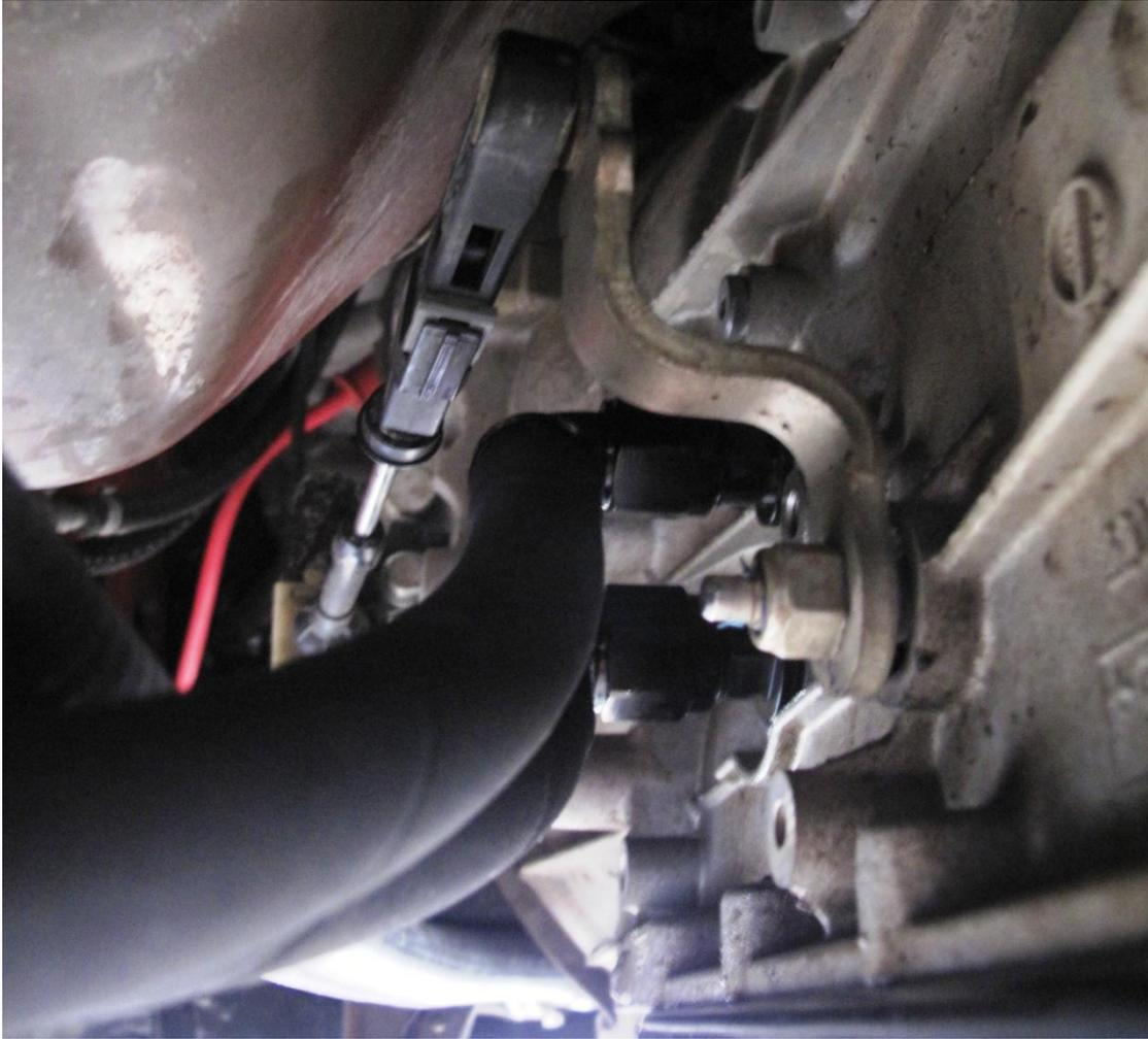
15. Re-attach the oil line retainer plate and tighten up the bolt using a 10mm spanner. Use the supplied zip ties to pull the hoses together and tidy up any slack. The line clamping tools can now be released.
