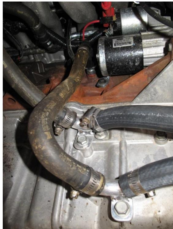
*(Note: For FG applications this shorter hose should be trimmed back to 635mm long for a perfect fit.)*
