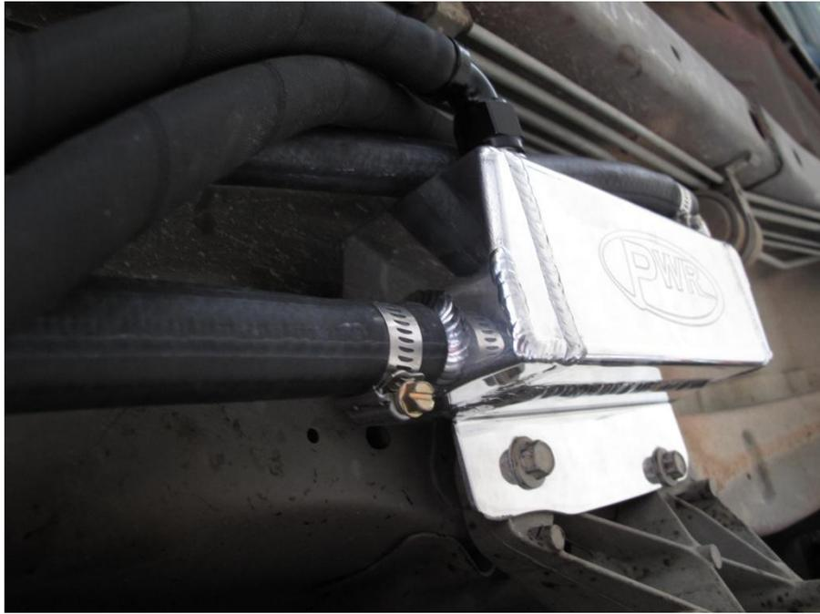
14. Ensure that the oil lines are above the heater hoses and press the adapters into the side of the transmission, noting that the longer hose goes into the top port of the transmission. Angle the hose ends downwards approximately 45° to allow adequate clearance around the shifter linkage, as shown below.
