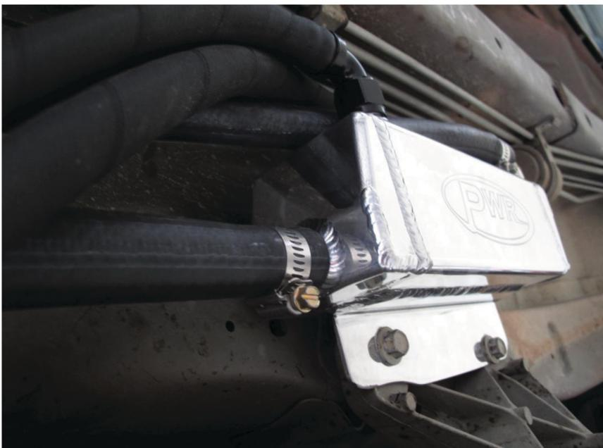
Ensure that the oil lines are above the heater hoses and press the adapters into the side of the transmission, noting that the longer hose goes into the top port of the transmission. Angle the hose ends downwards approximately 45° to allow adequate clearance around the shifter linkage, as shown below.
