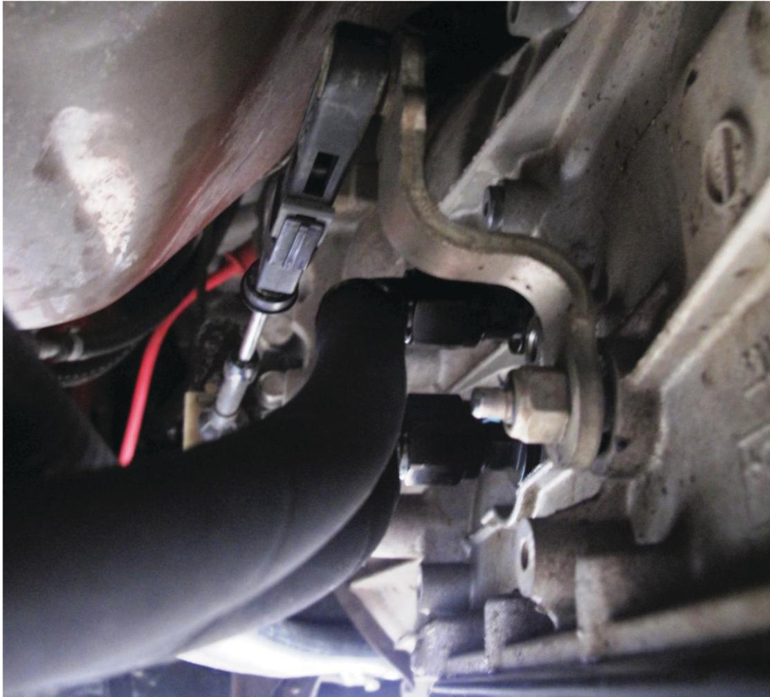
Re-attach the oil line retainer plate and tighten up the bolt using a 10mm spanner. Use the supplied zip ties to pull the hoses together and tidy up any slack. The line clamping tools can now be released.
