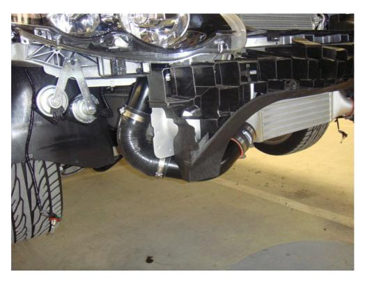
Connect Pipe Item **No.6** and Item **No.7** placing a 2.5 hose clamp on each as pictured . Keep in mind to align the hose clamps for ease of access to tighten. Tighten each clamp.
