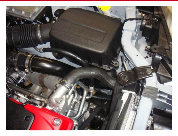
Fit silicon hose No.12 to end of pipe entering engine bay (pipe item No.11)
