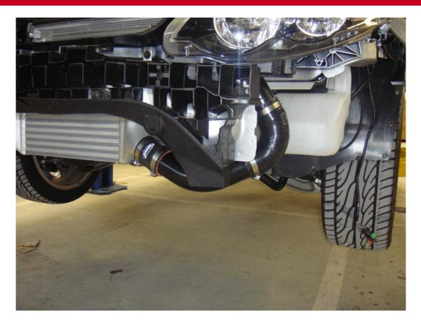
Working our way to the left side of vehicle, proceed to feed item no.11 though under head light and leave hang there.
