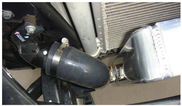
Proceed to refit clamps and tighten, proceed to secure the passenger side hose clamps also.
