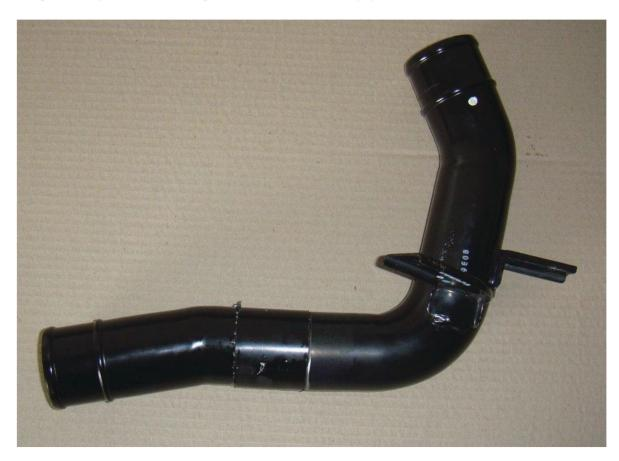
With a rag, mount this pipe in a vice and proceed to cut approx 140mm off the pipe, leaving 40mm remaining of flared section. Remove any sharp edges or debris from the cut.
