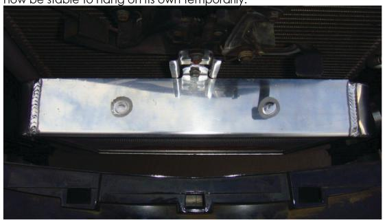
Proceed to align the 2x bottom mount holes with the factory chassis mount points, using 2 x m6 bolts from the original equipment Intercooler. Ensure the intercooler is level prior to fully tightening.
