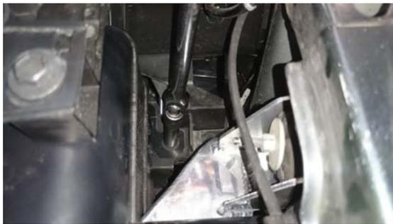
42. The lower 2 screws require the T-25 Torx driver.
