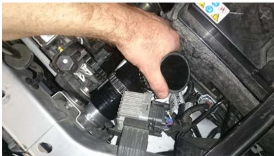
2. Push the 67-degree lower silicone bend on to the intercooler first then push on the 2.25 – 2.5 inch silicone at the throttle body end of the pipe.
