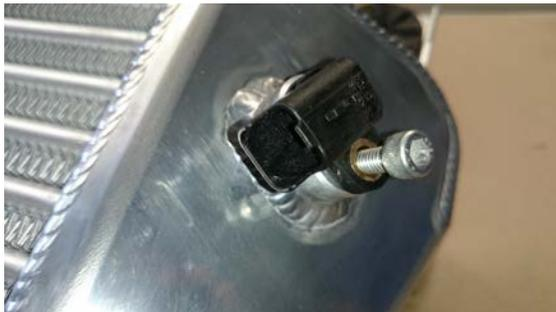
29. Taking care not to damage the core install the new intercooler paying attention to making sure the lower foam strip is in contact with the radiator core support as per next image. Using the original nuts and bolts secure the intercooler into place.
