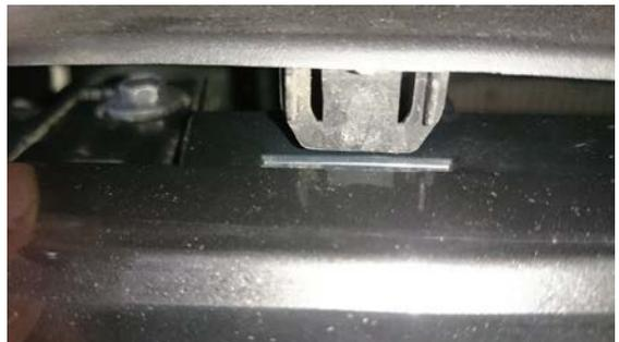
6. Remove the grille retaining bolts using a 10mm socket. There are two bolts on each side. One at the top and one deep next to the head light behind the air duct. Retain for reinstallation.
