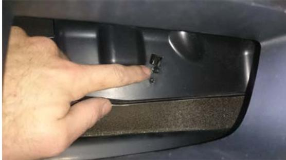
34. Reinstall the front bumper being sure to clip in under the head lights firmly.
