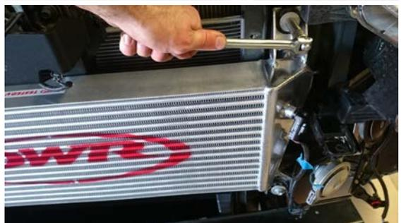
30. The supplied spacers (99A18985) may need to be placed behind the intercooler to ensure adequate clearance of approximately 3mm from the Intercooler core to the radiator core support panel area as highlighted in images below with arrow.
