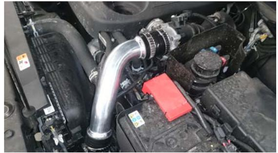
4. Remove hot OEM hose as per step 18 and 19 in section 1. Ensure that you have removed any tape or rags from inlets and outlets
