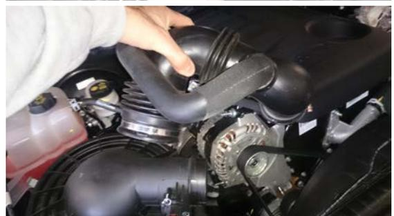
19. Undo and remove the bottom intercooler inlet hose again by undoing hose clamps.
