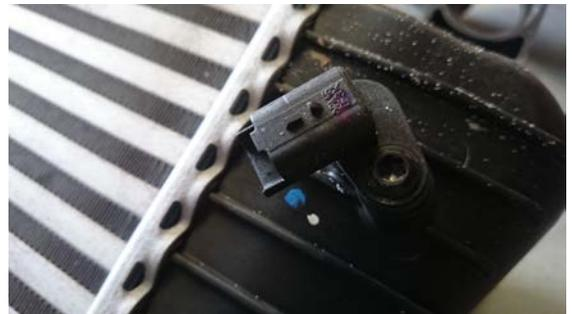
26. Remove the rubber mounting grommets from the OEM intercooler and place aside for reinstallation into the new PWR intercooler.
