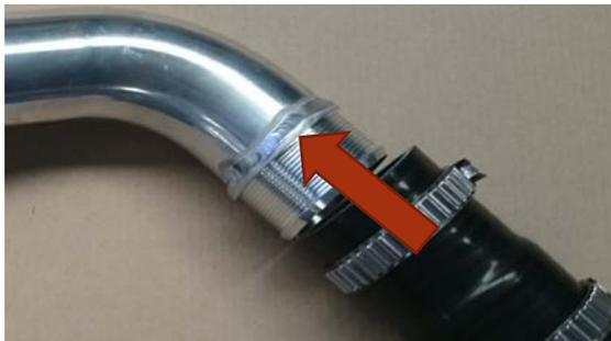
3. Be sure to push the silicone all the way on to the pipe up to the shoulders. Once in place tighten firmly and check it is secure and will not rub on anything.
