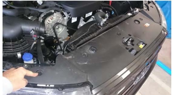
10. Connect battery and confirm that all hoses, pipes, wires and panels are secure. Ensure that no tools or obstructions have been left under the bonnet and your PWR Intercooler and pipe kit is now installed.
