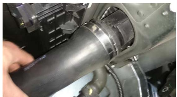
20. Undo and remove the radiator air ducting (2 places each) using an 8mm socket and retain for reinstallation.
