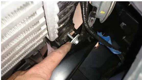
24. Remove intercooler and place aside for disassembly.
