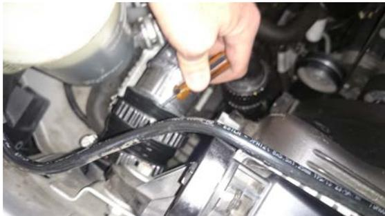
7. Again push all hoses up to the shoulders of each outlet firmly and tighten clamps. Check all hose clamps are tight.
