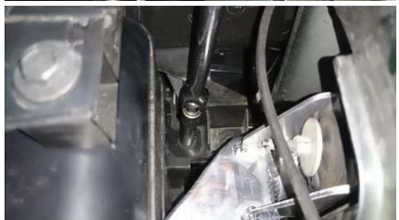
7. Using a T-25 torx bit undo the 2 screws at the bottom of the grille retaining it to the bumper.
