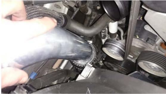
6. Next push the top of the aluminum pipe into the hump hose on the intercooler. It is best to guide the bottom edge of the pipe into the silicone first and then slide the top edge of the silicone over the pipe outlet. Using caution, you may want to use a small flat screw driver to lever as per picture below to allow the hose to slip on easier. These pipes are a very snug fit to avoid any blow off under high boost applications.
