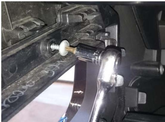
43. Once the grille is secured move onto the top trim panel. The trim panel is to be clipped in into the grille then using the 5 original push pins lock it into place.
