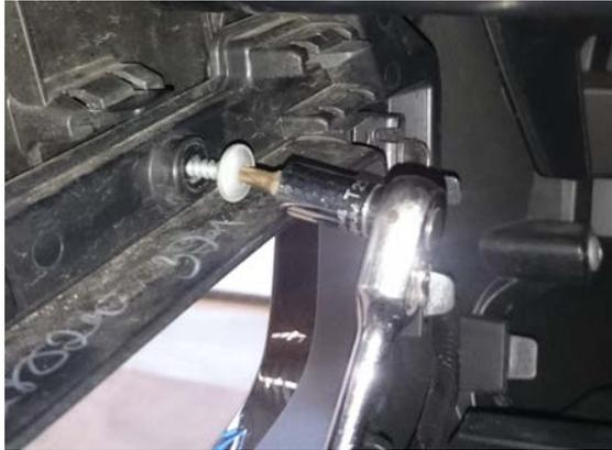
8. Carefully release all the clips holding the grille to the bumper 4 of the clips need to be reached from under the car while the rest can be reached from the engine bay.
