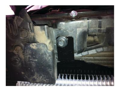
The  $2 \times 3/8$  Trans Lines can now be run off the transmission cooler off to the right around the side of the radiator and to where the 2 main lines run to the factory in tank transmission cooler. The line directions are marked below. Secure lines with zip ties as you go.
