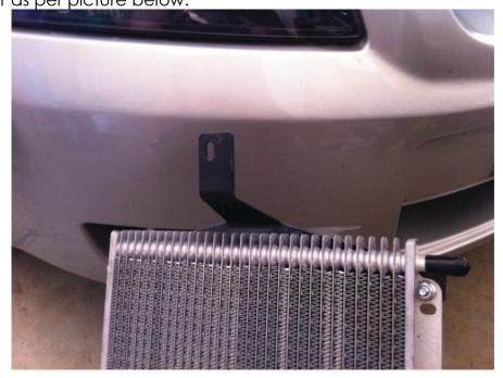
The assembled Transmission cooler and top bracket can now be slid in from the lower bar opening, you may need to push the condenser and
