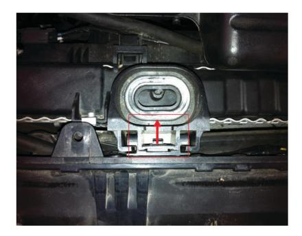
Now with the top mounts released, push the radiator and condenser assembly back towards engine to give easier access to the top 10mm condenser mounts, remove the LH and RH bolts to separate condenser from radiator. Now coming in from the lower opening in the front bar, the condenser can be lifted out of its mount holes.
