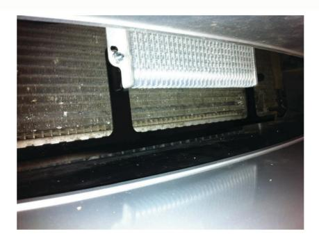
Now is a good time to assemble the top bracket to the Transmission cooler as per picture below.
