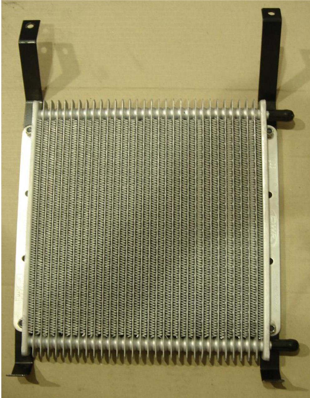
From the top grille opening, lower the PWR transmission cooler into place, slightly off set to the drivers side (transmission cooler outlets pointing to the passenger side of vehicle) until the hole in the drivers side bracket aligns with the existing far hole nearest to drivers side headlight. Proceed to drill a 6mm hole in the opposite top mount bracket and secure with M6 bolts & nuts supplied.
