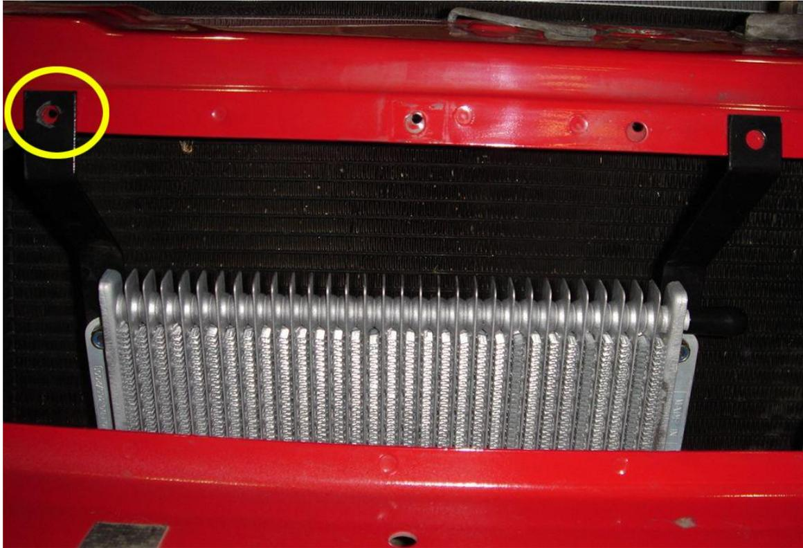
With the top of PWR cooler brackets now secure, proceed to drill a pair of 6mm holes to align with the lower bracket holes as circled.
