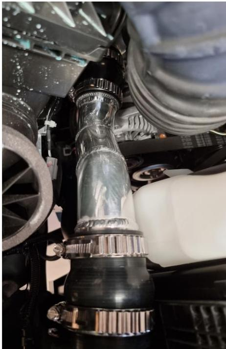
29. With Plastic engine cover removed, loosely fit the cold pipe onto the intake manifold of the engine with the other end close to the opening on the passenger side of the radiator
