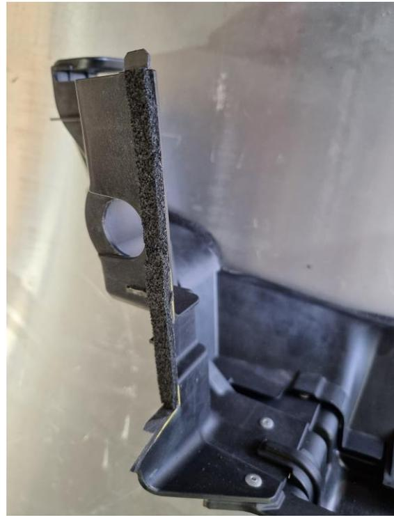
23. Remove the bonnet latch sensor harness clip from the harness as shown. There isn't sufficient clearance with the harness clip attached to the bracket once the PWR Intercooler is fitted. A zip tie is supplied to hold this wire in place upon reassembly.
