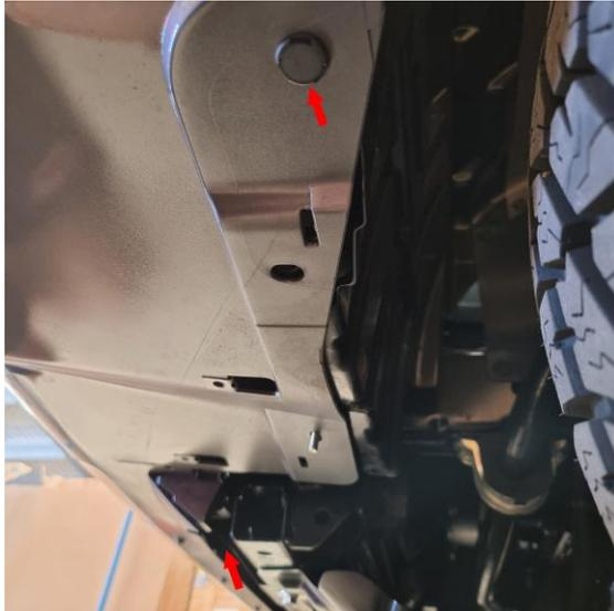
9. Remove 4 x small scrivets inside each wheel arch area carefully, as these are prone to breaking easily.
