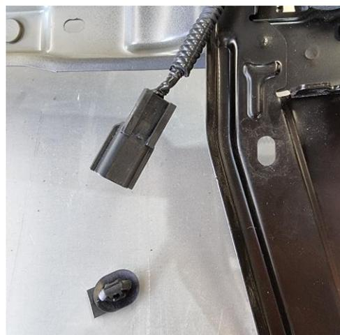
24. The harness bracket on the passenger side of the bonnet latch support needs to be bent to allow clearance. A small cut (indicated by yellow line) will allow this to bend flat as shown.
