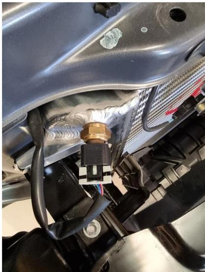
17. Loosen all 4 hose clamps on hot and cold side intercooler hoses. Remove top 2 x nuts and lower 2 x bolts on intercooler. The intercooler can now be removed. Remove hoses if hard pipe kit has also been purchased. Press out steel inserts before removing rubber bushes from OEM Intercooler to be reused.
