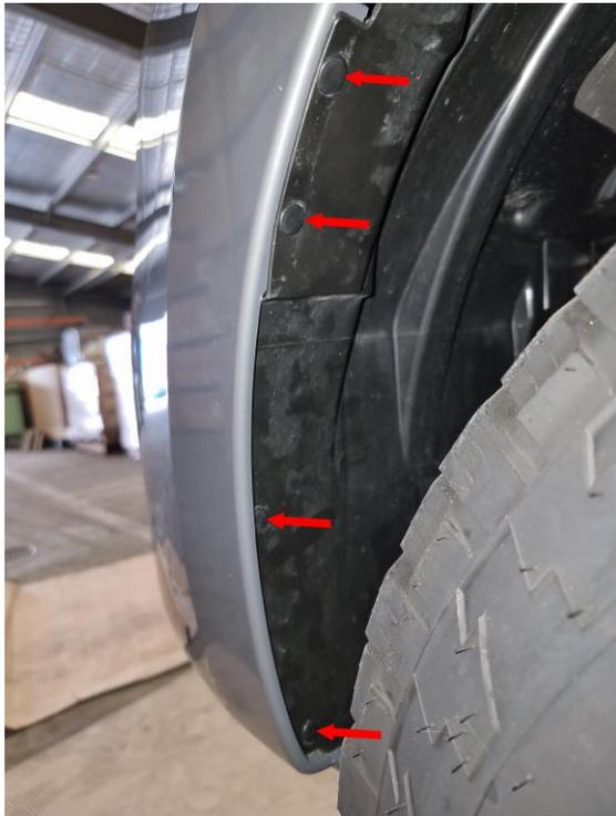
10. Move the passenger side wheel arch liner away from the bar enough to gain access to inside the front bar to release both wiring harness connectors with a narrow flat blade
