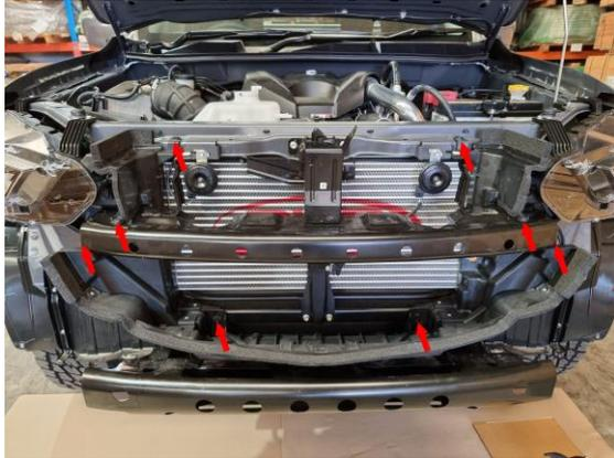
14. Remove front bumper bar support by removing 6 x nuts and 2 x bolts securing the headlights. Unclip sensor before removing.
