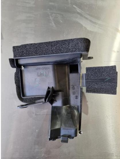
21. On the lower plastic ducting, if the self adhesive foam is in good condition, it can be carefully peeled back and re-used against the new cut edge on the next step.
