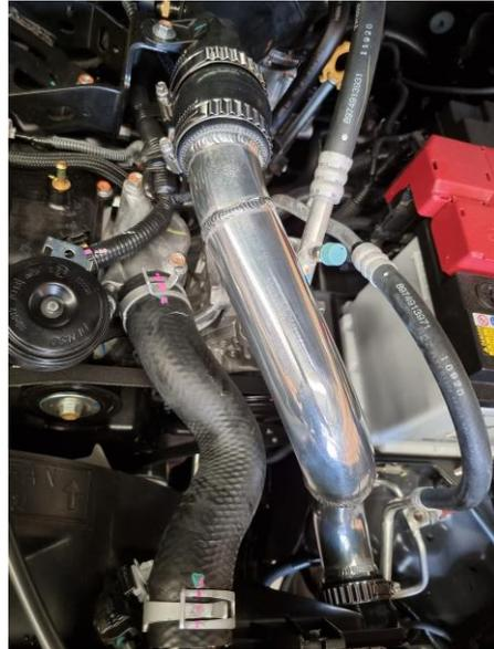
30. Slide the intercooler into position onto the upper studs on the radiator support panel whilst ensuring that the silicone hoses are going onto the intercooler outlets on both sides, otherwise intercooler won't fully seat into its final position.
