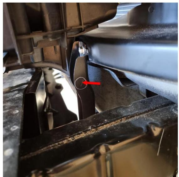
13. Remove 8 x scrivenets securing both upper driver side & passenger plastic ducts and entire lower plastic duct. The ducts can all be removed.
