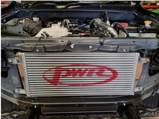
16. Remove white clip from temperature sensor to allow the harness to be released and remove sensor from OEM Intercooler to be refitted to your PWR Intercooler.
