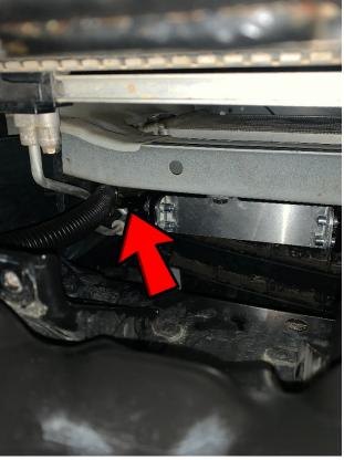
Step 9: Now you will turn the inlet of oil cooler up and fill the cooler and lines through this barb. We recommend adding roughly a litre of fluid.
