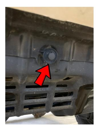
Step 4: Once the underbody protection has been removed you will remove the below transmission line using pliers to release the clamps.
