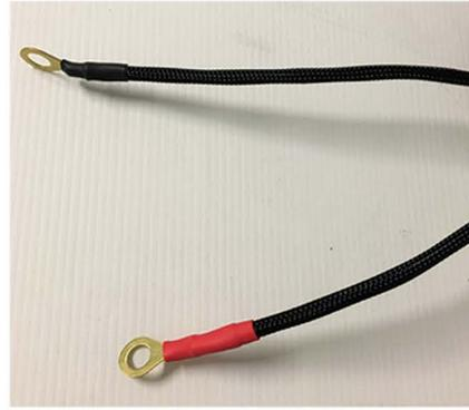
1. Connect the 8mm eyelets to the battery posts.
