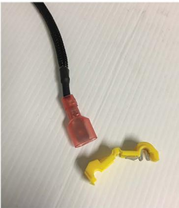
6. Clip the yellow EZ tap connector onto the white wire in the 4 plug.
