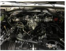
Remove the two factory flange gaskets.
