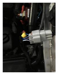
Use the supplied EZ Yellow clip by opening the clip, place it over the white wire as indicated, close the clip until it locks. Insert the EZ clip into the connector as shown below.
