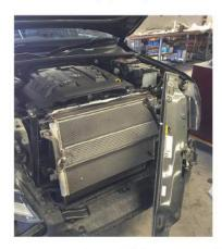
27. Remove the visible screws holding the air condenser, intercooler and transmission cooler in place.
