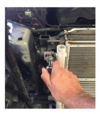
Unscrew screws holding the air condenser and transmission hard lines in place.
