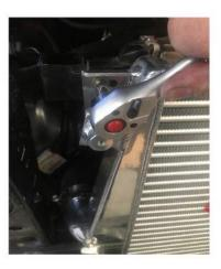
47. Click on the factory sensor plug on the bottom passenger side outlet.
