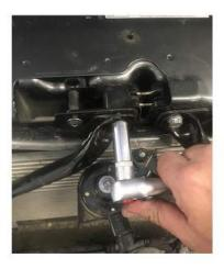
61. Mount the front intrusion bar using the factory bolts.
