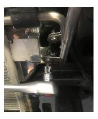
56. Tighten the M6 hex head bolt with a open end spanner on the trans cooler mount.
