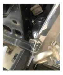
55. Refit the 2 factory bolts to the transcooler lines bracket on the passenger side.
