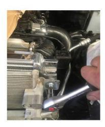
53. The driver's side mount requires the use of the PWR supplied billet spacer, 32mm M6hex head bolt and big washer..
