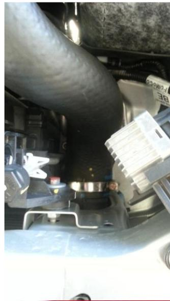
4. With the 10mm long ratchet socket, remove the upper and lower bolt retaining the driver's side intercooler air duct. Then remove the small retainer scrivet also located on the duct. Repeat this for the passenger side. Remove both ducts.
