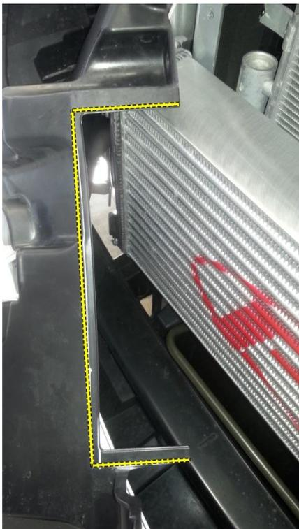
16. With the intercooler secure and bar brackets refitted, we now need a sharp blade or hacksaw. You will need to trim approximately 5mm off the front edge, 5mm off the top and 8mm off the bottom of the plastic air ducts, as shown to the left.
