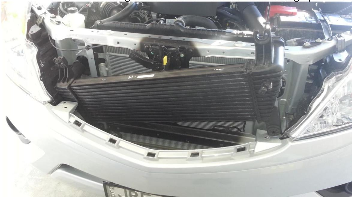
10. While the intercooler is out, using the T27 Torx bit, loosen and remove the intercooler air temp sensor retainer screw. Carefully remove the air temp sensor. Place this sensor into the new PWR intercooler billet sensor boss and tighten the sensor with the 5mm Allen key bolt provided with the cooler.
