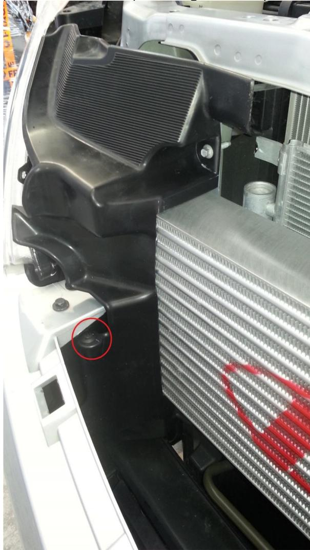
19. Reaching over into the engine bay, proceed to fit both boost air pipes to the intercooler. This will be a tight fit, as the PWR unit is 2mm larger in diameter compared to the original, just to ensure a secure seal. Tighten clamps firm.
