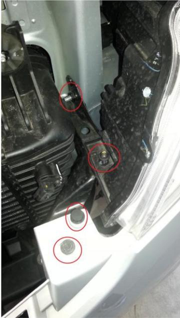
8. Repeat step 7 on the passenger side, including the same 12mm bolt that is only accessed from the wheel arch.
