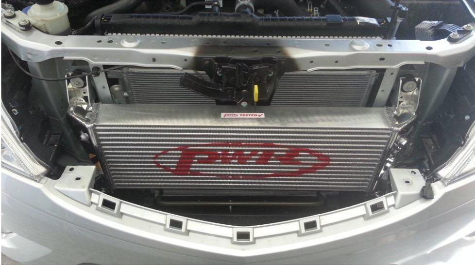
13. Locate the intercooler onto the top mounting studs and proceed to tighten the 12mm nuts and then tighten the lower 12mm bolts.
