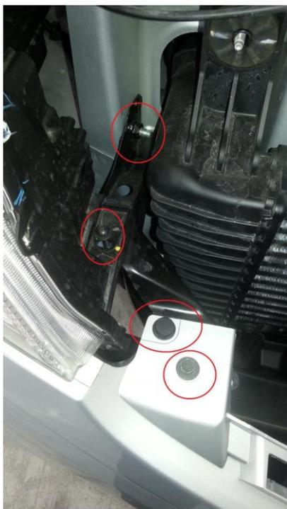
7. Remove both RH and LH Bar / headlight brackets. With the 10mm socket, loosen and remove the bolt. Using the flat blade screwdriver, raise the scrivet head and remove scrivet. With the T27 Torx bit, loosen and remove the long screw. With the 12mm long socket, loosen the 12mm bolt inside the engine bay. There is a second 12mm bolt underneath this, that is reachable only from under the car. Loosen and remove both of these. Then remove the bar bracket completely.
