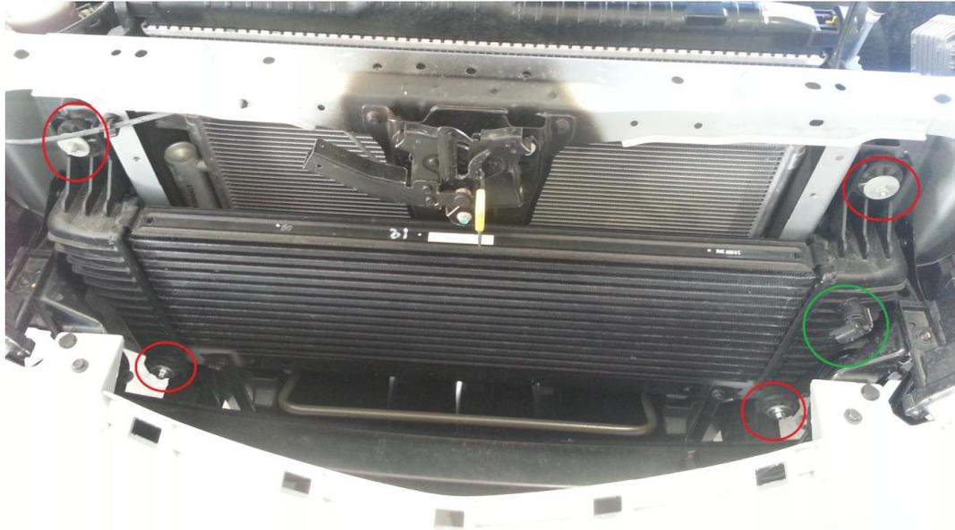
6. Remove the 4 mounting nuts washers and rubbers circled in red with the 10mm long socket (circled in red above) Leave the intercooler sitting on the top studs for now.
