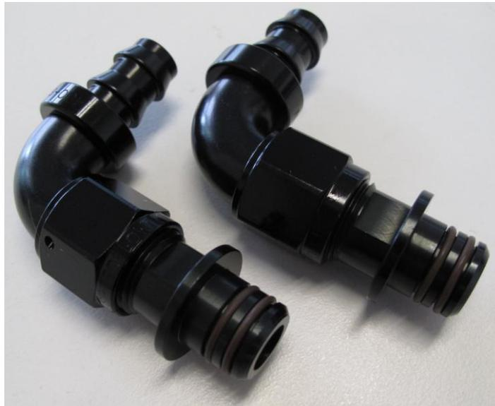
Attaching the hoses onto the PWR Heat Exchanger is best done off the car, due to the tight confines when mounted. The longer oil hose is to be tightened onto the top fitting and the shorter hose is tightened onto the lower fitting using a 7/8" spanner, ensuring the hoses are parallel to the heat exchanger.
